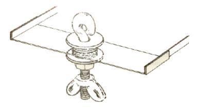
When adjusting the suspended masses to swing with the tray, it is critical that they do not rub. Any rubbing will cause the swings to decrease too rapidly for proper determination of the frequency
