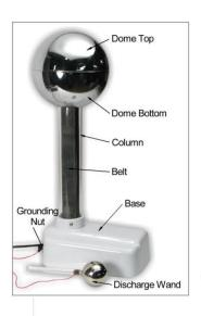
Tabletop versions of the VDG generator range in size from several feet tall producing half a million volts, down to tiny 2-inch versions which produce only five thousand volts. Physics researchers use larger ones, some of which are several stories tall and produce many megavolts output voltage.
